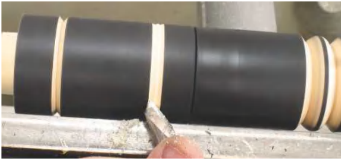
▲ Pic.7 Now the tool is making a cut on the other side, only take small amounts of material from each side until the cove gets wider
